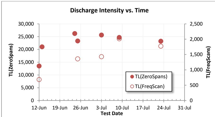
Figure 3 Plot showing the discharge trend of the red phase of the 35kV transformer bushing.
