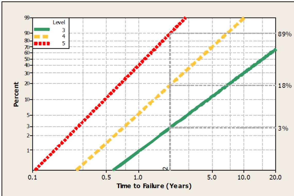
Figure 12. Diagnostic performance curves for one on-line PD test technique.
