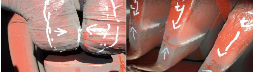
**Figure 9 Discharges between phases in the form coil bars and PD from the grading coating.**
