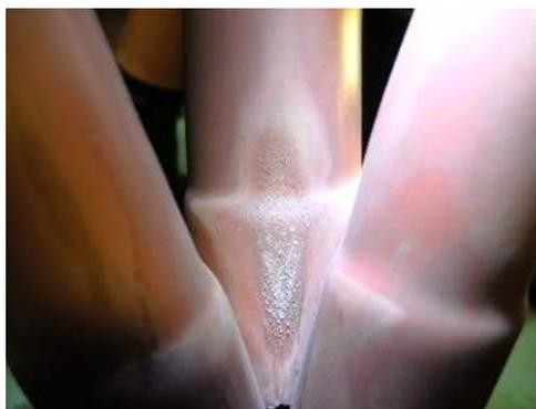
**Figure 8 Discharges in one phase of the trifurcator.**
