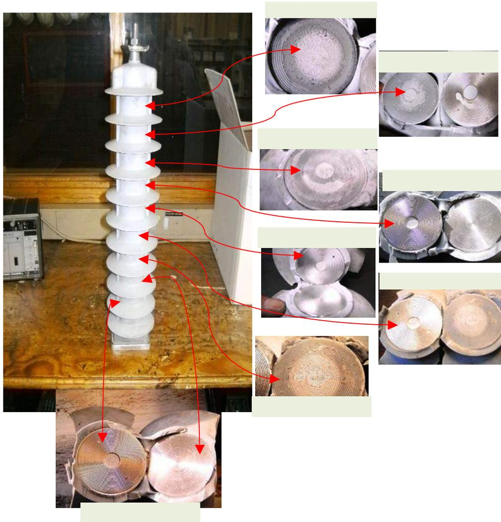
**Figure 10. Discharges in a faulty gap arrester.**
